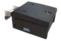
Desktop compact thermal printer able to print an additional barcode on parking tickets collected at the entry station. These barcodes, read by the ESPAS30-P automatic pay station, are identified as bonuses, allowing the application a discount in terms of price or minutes when calculating the tariff.
